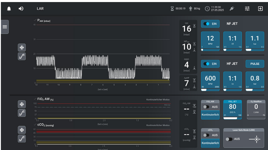
Fig. 12: Basic settings of the ventilation parameters for supraglottic SHFJV – TwinStream EVO display
